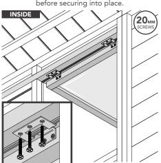
Secure the Casement Stay & Pins to the Window and interior sill. Secure the Casement Stay with its supplied screws and use it to position the pins underneath. Mark out first to ensure they align.
