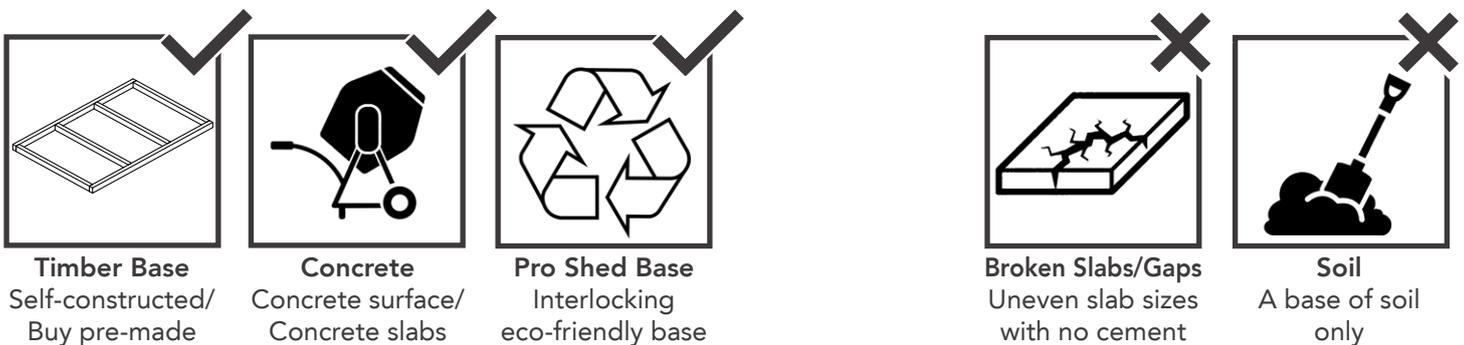
If you have an existing base and think it's suitable for your new shed to be sited on, it is important you check that it is level and doesn't deviate by any more than 15mm from edge to edge. If this isn't the case the building will twist, causing gaps to appear in the sections and the roof, doors and windows to misalign.
