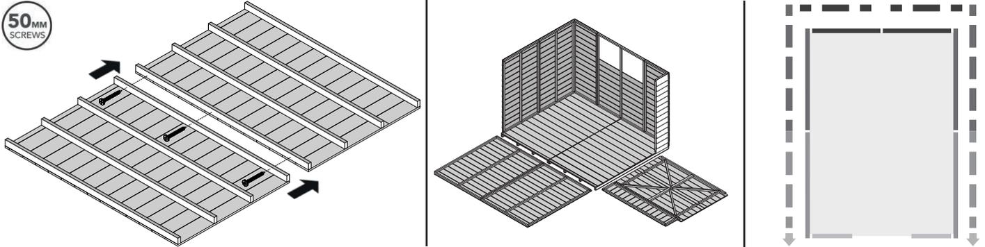
**1b** Start at a back corner. See the section layout on page 4 to confirm position. Secure the corner as shown below.
